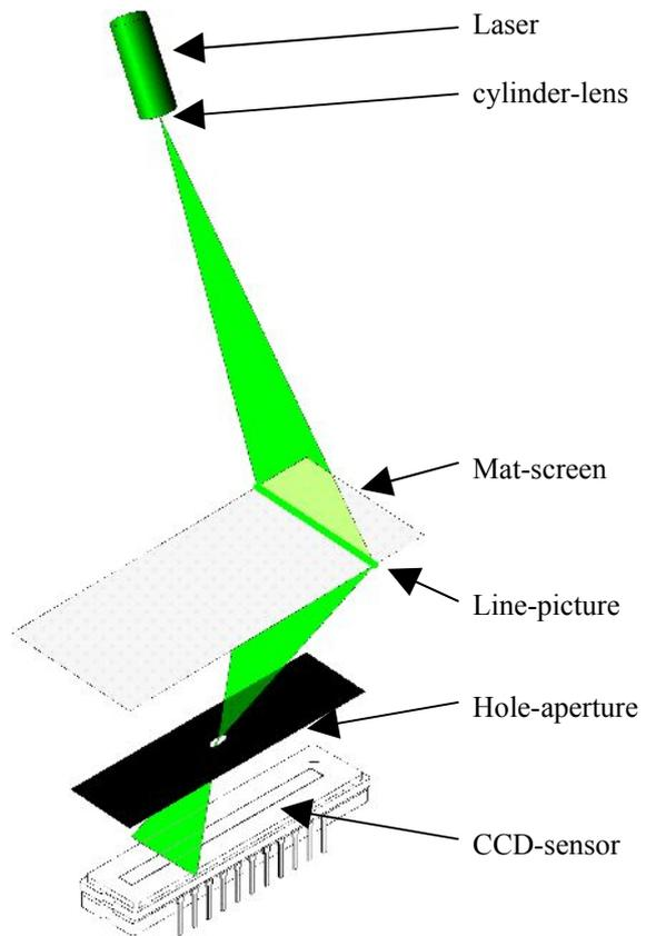
**Figure 6: Schematics of the optical path**
