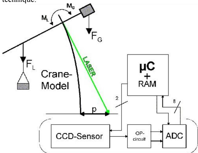
**Figure 5: Sensor parts and its components**
